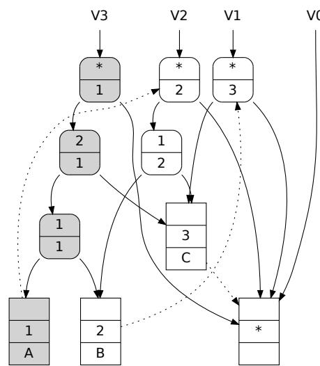
Figure 4.2: **A persistent Directed min-tree** is created by referencing the root of a version from the leaf of the past version from which the path was copied. In this example each leaf is linked to the version of the data structure from which it was created by path copy. The links from the leaves to the roots are dotted and the most recently created path is shaded. The Immutable Data Structure is persistent because past versions are accessible by a look-up function which follows these links.
